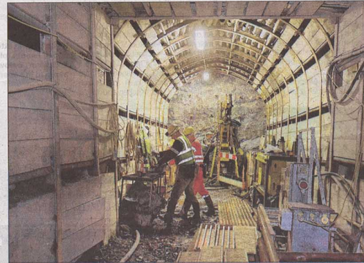
■ Some 350ft below ground, miners work the diamond drill to collect rock core.
