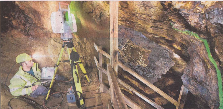
■ The business end of operations at South Crofty – surveying by laser scanning is undertaken through the mine workings.
